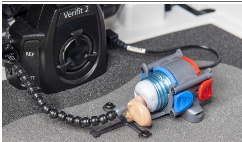
Positioning a ITE instrument for ANSI tests
