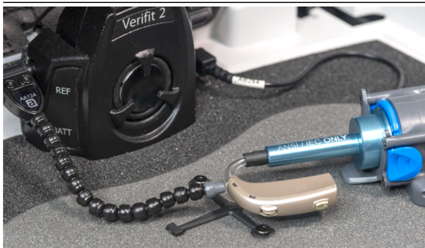
Positioning a BTE instrument for ANSI tests
