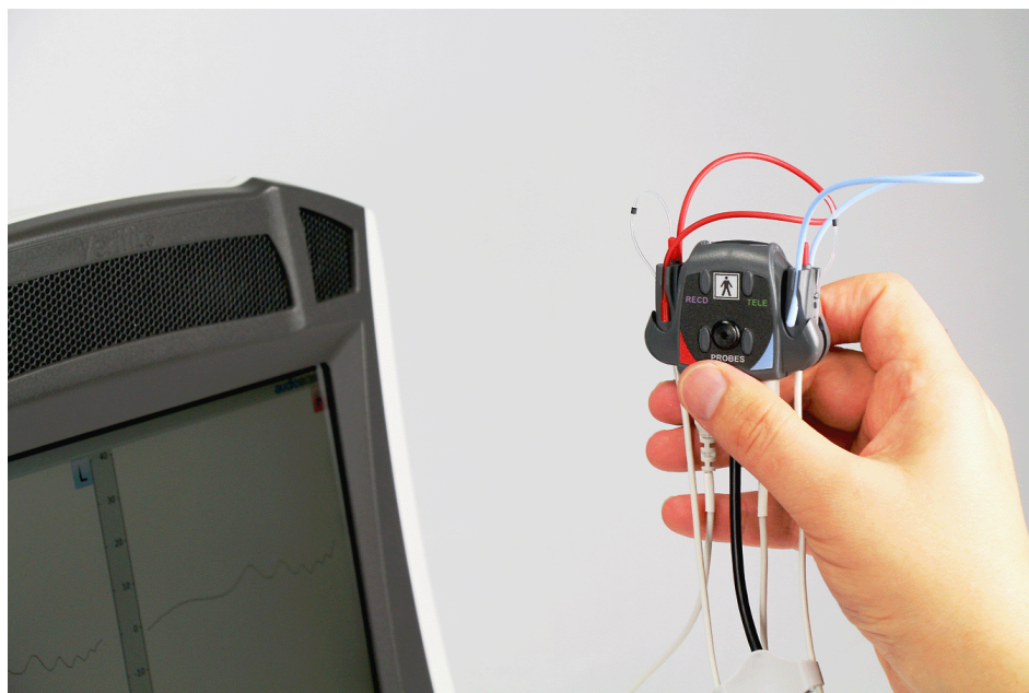
Hold probe dock with microphone to be calibrated facing speaker.
