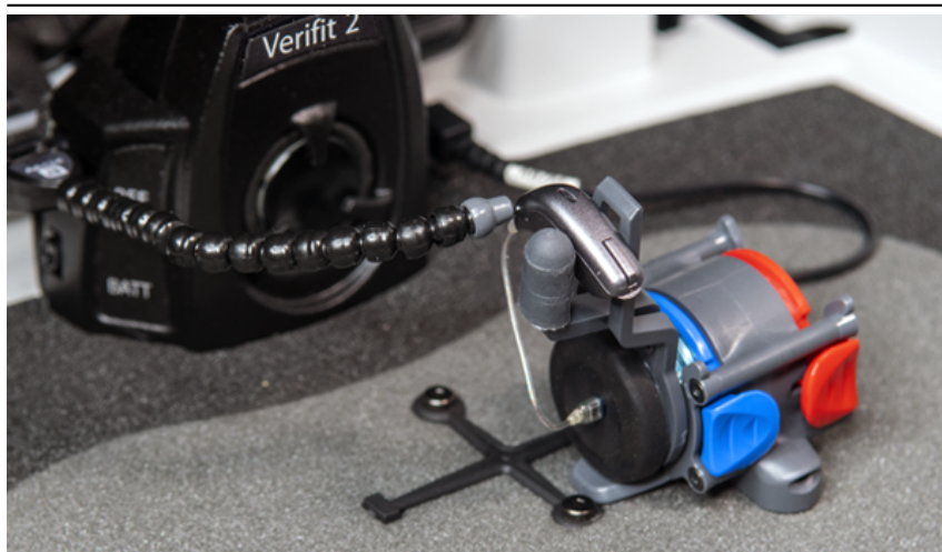
Positioning a RIC instrument for ANSI tests
