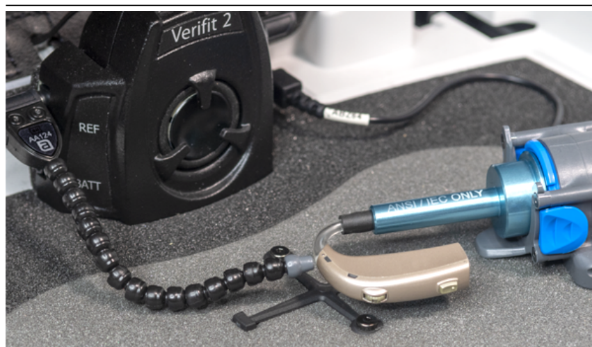
Positioning a BTE instrument for ANSI tests
