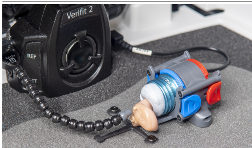
Positioning a ITE instrument for ANSI tests
