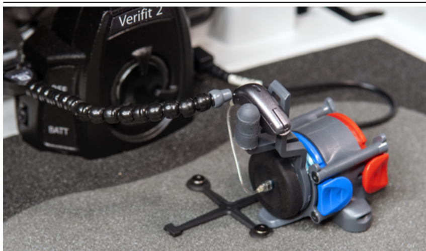
Positioning a RIC instrument for ANSI tests
