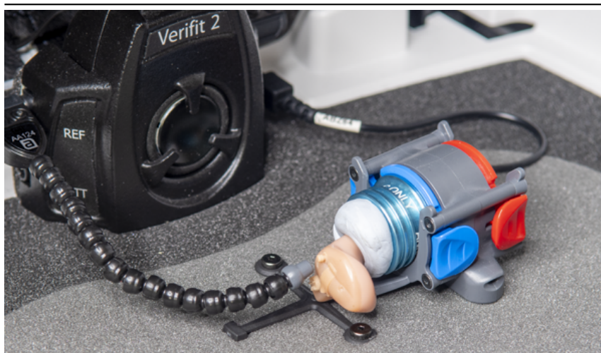
Positioning a ITE instrument for ANSI tests
