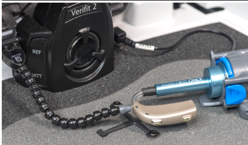
Positioning a BTE instrument for ANSI tests
