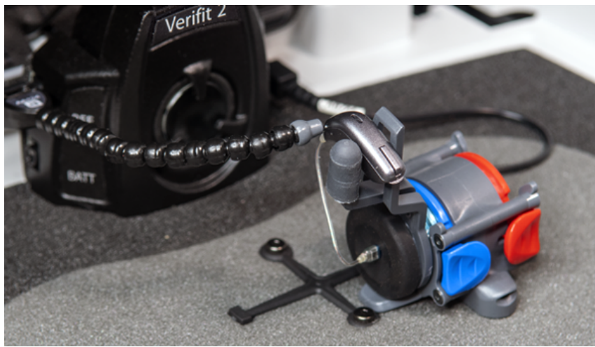
Positioning a RIC instrument for ANSI tests
