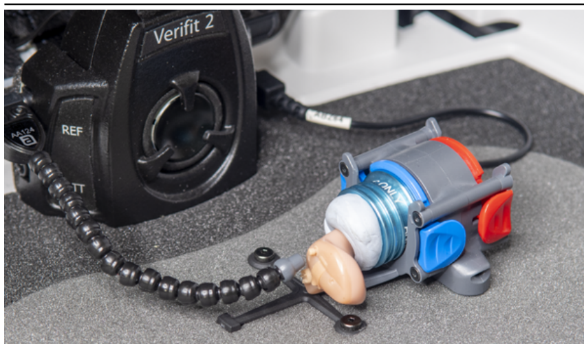
Positioning a ITE instrument for ANSI tests
