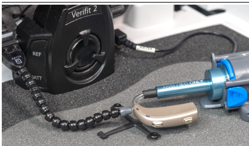
Positioning a BTE instrument for ANSI tests
