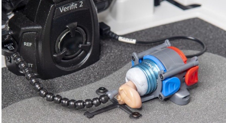
Positioning an ITE instrument for ANSI tests
