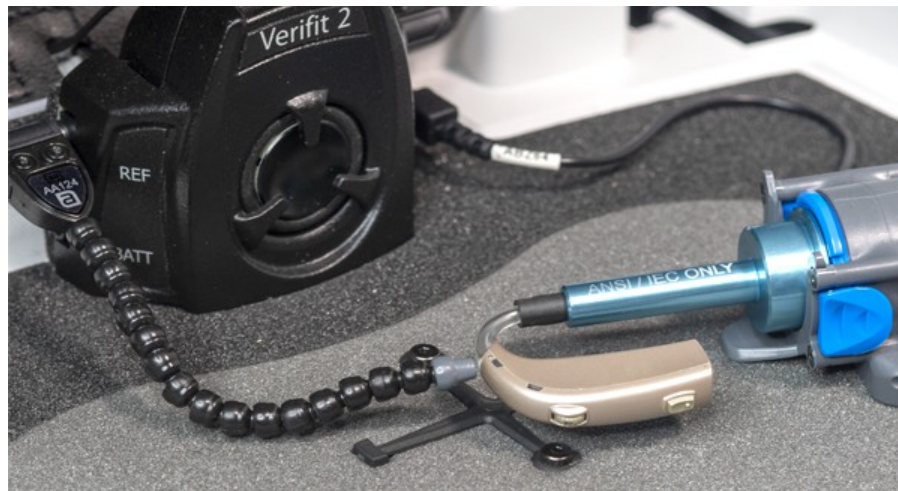
Positioning a BTE instrument for ANSI tests
