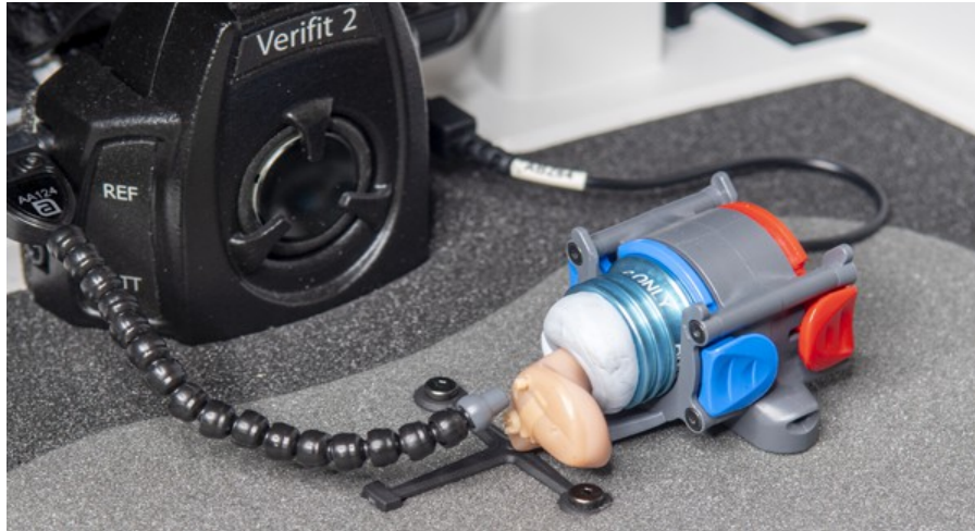
Positioning an ITE instrument for ANSI tests
