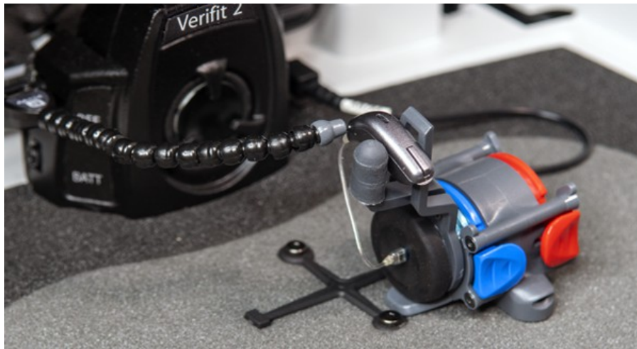
Positioning a RIC instrument for ANSI tests
