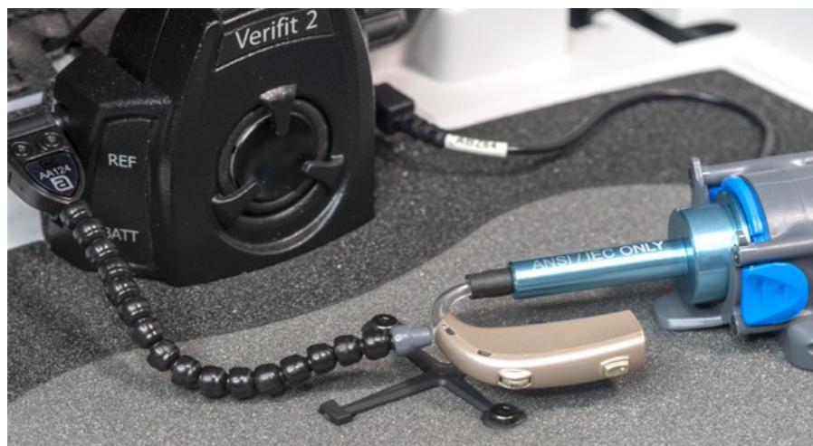
Positioning a BTE instrument for ANSI tests
