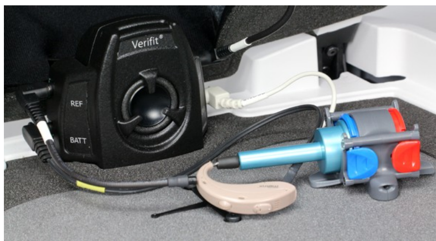
Positioning a BTE instrument for ANSI tests
