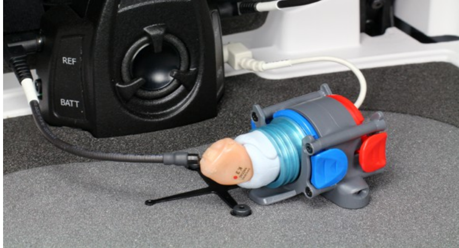
Positioning an ITE instrument for ANSI tests
