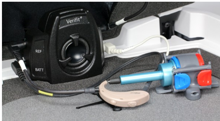
Positioning a BTE instrument for ANSI tests
