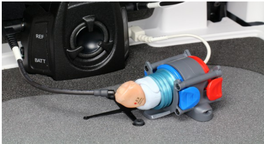
Positioning an ITE instrument for ANSI tests
