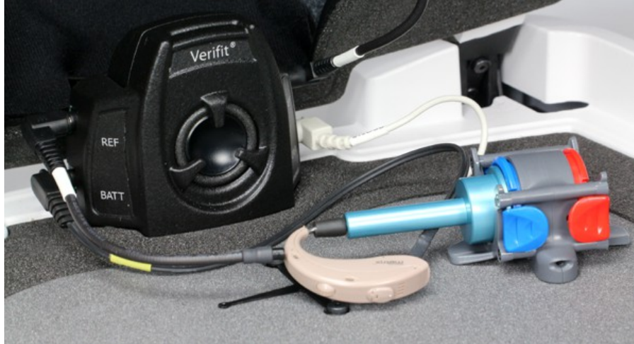
Positioning a BTE instrument for ANSI tests
