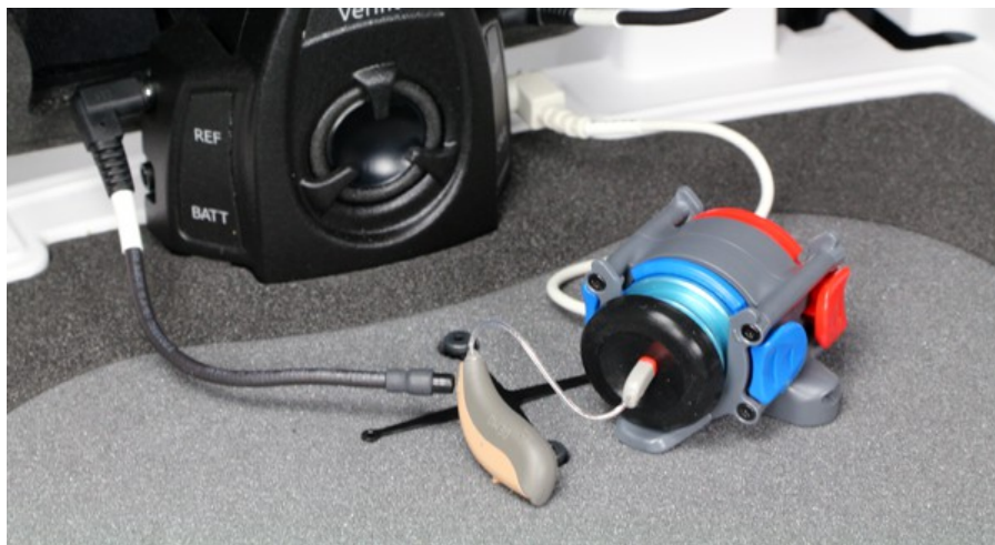
Positioning a RIC instrument for ANSI tests
