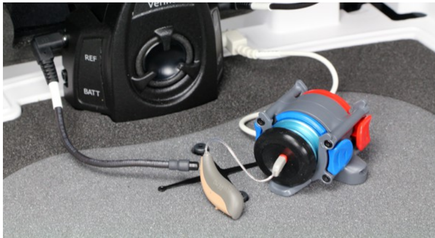
Positioning a RIC instrument for ANSI tests
