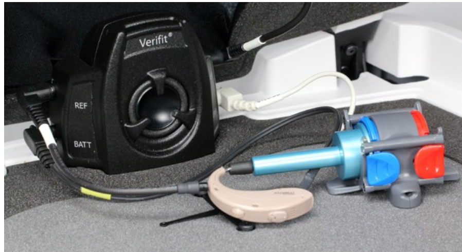
Positioning a BTE instrument for ANSI tests
