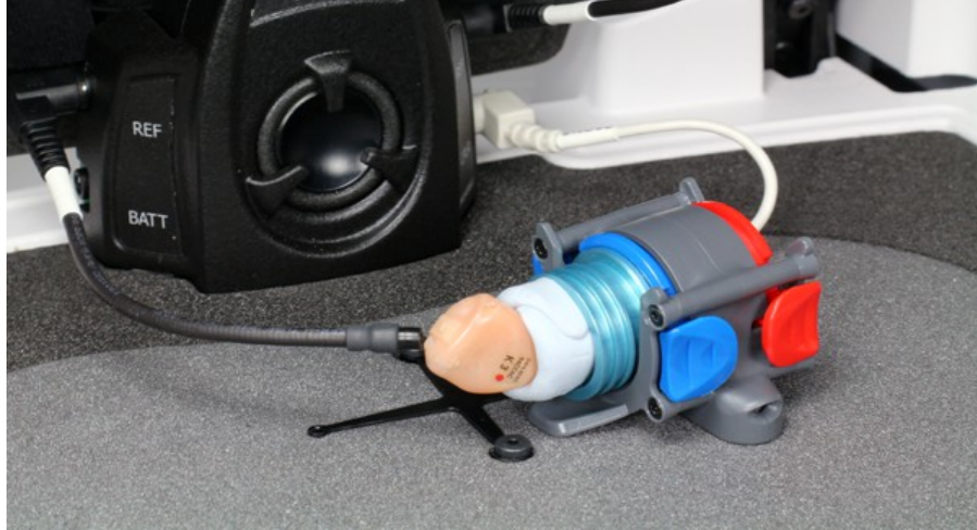
Positioning an ITE instrument for ANSI tests
