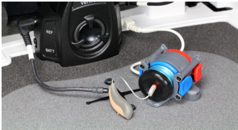
Positioning a RIC instrument for ANSI tests
