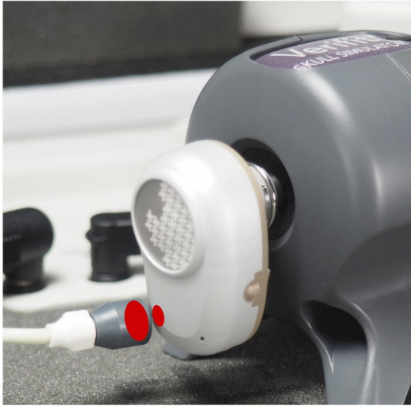
Left-ear device reference microphone position
