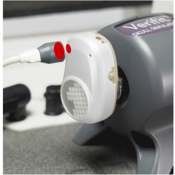
Right-ear device reference microphone position
