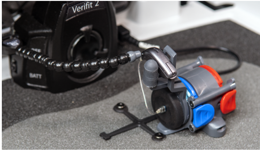
Positioning a RIC instrument for ANSI tests
