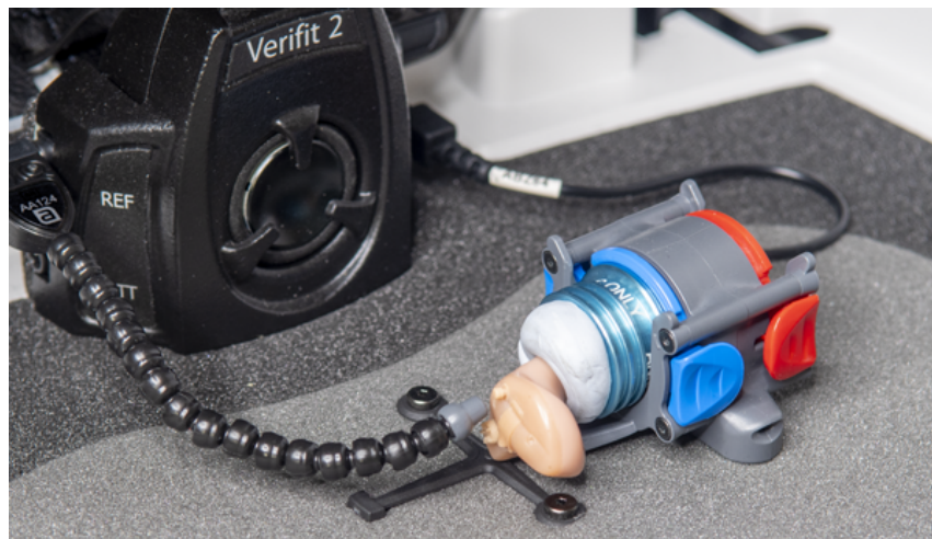
Positioning an ITE instrument for ANSI tests
