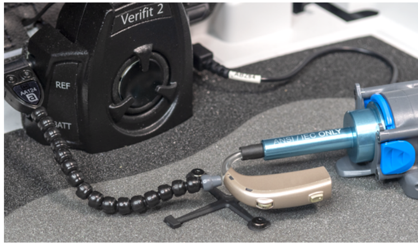
Positioning a BTE instrument for ANSI tests
