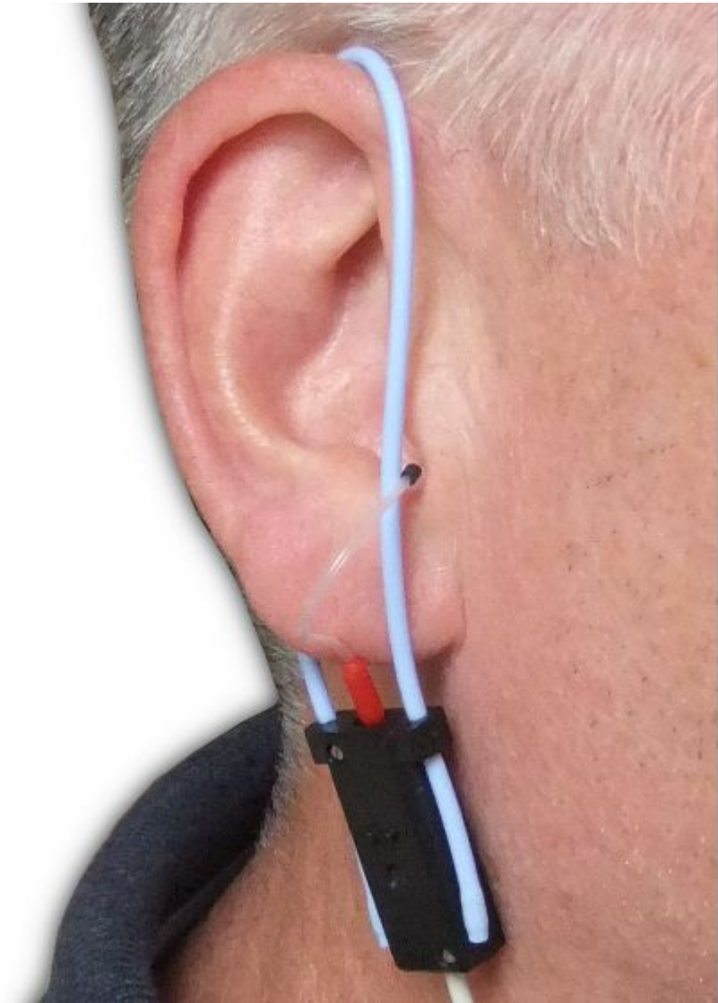
Probe tube insertion: The blue lanyard holds the tube in place and the depth marker is at the intertragal notch
