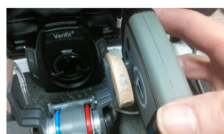
Figure 4. Positioning of the tele-test handset during coupler-based telecoil verification.
