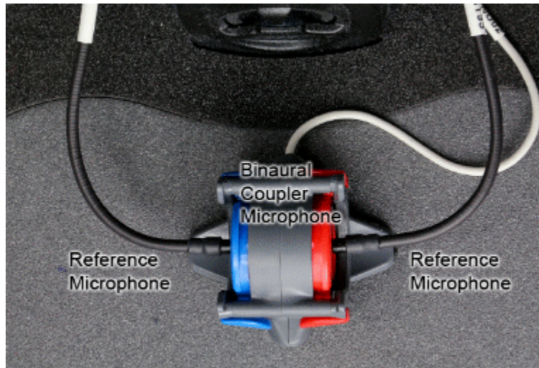
Test box reference microphone calibration position
