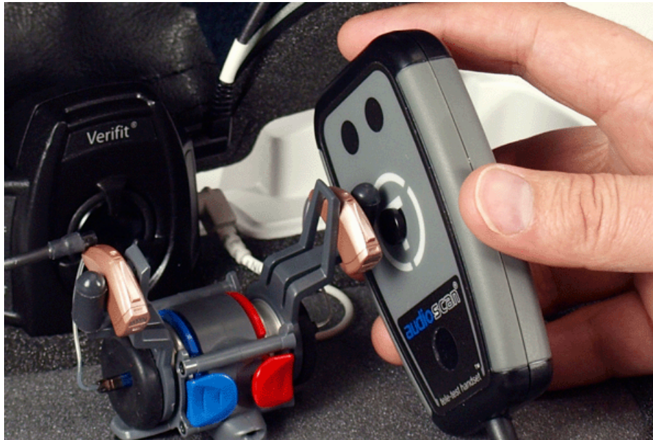
Tele-test handset position for Test box
