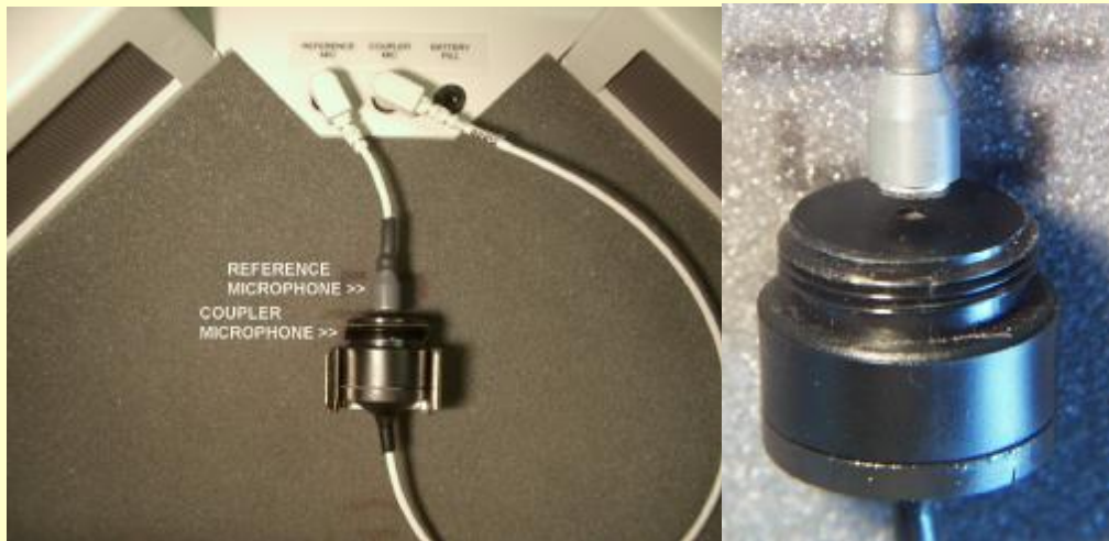
FastFacts 7.9: Calibration of test box reference microphone
