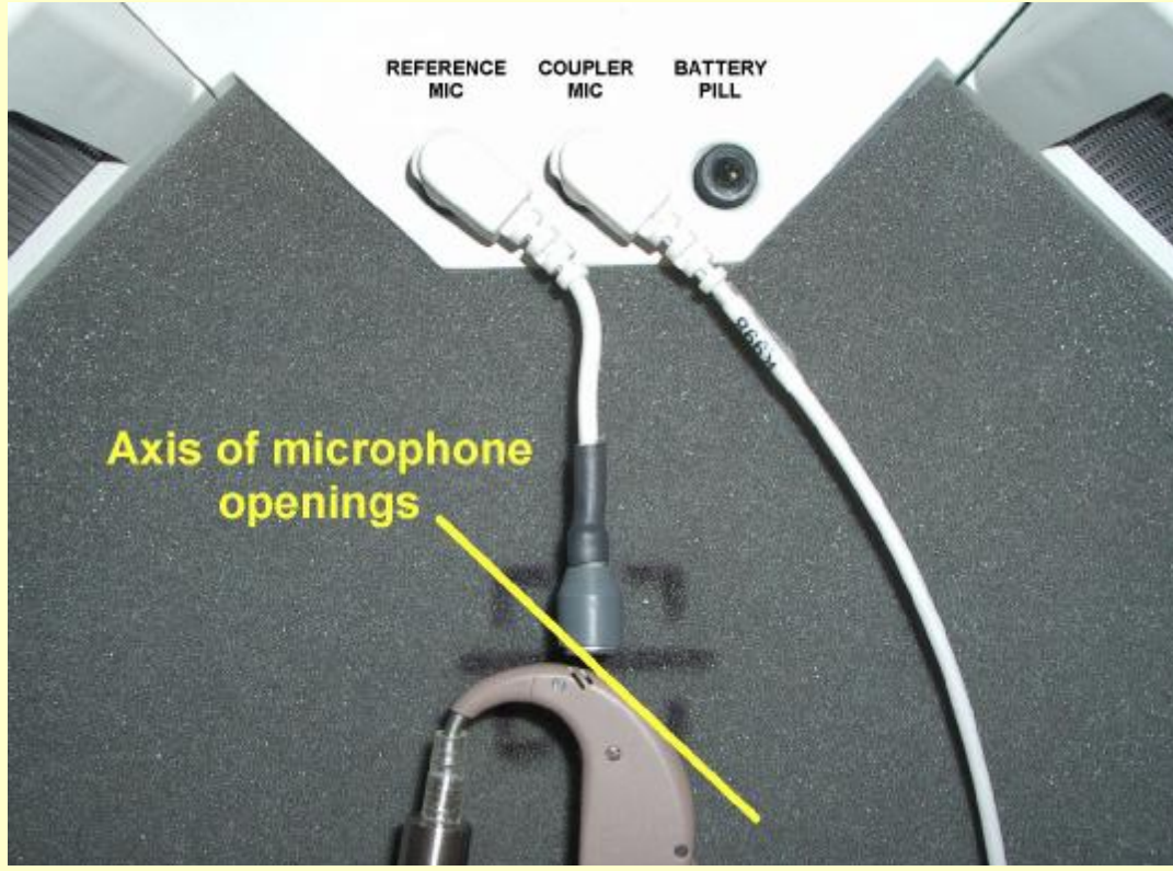
FastFacts 9.7: Directional BTE positioning
