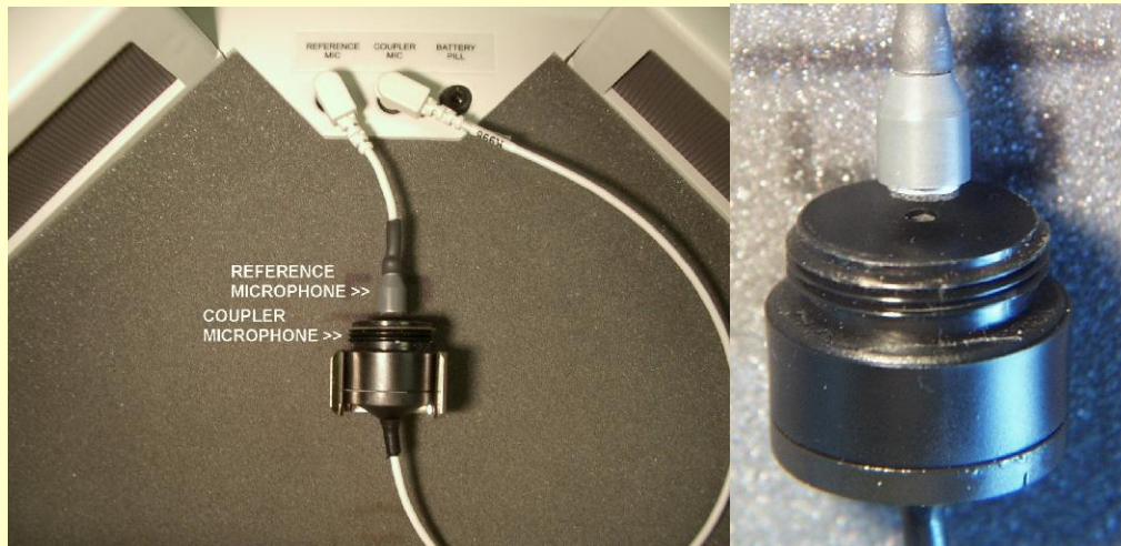
FastFacts 7.9: Calibration of test box reference microphone
