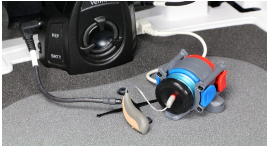
Positioning a RIC instrument for ANSI tests
