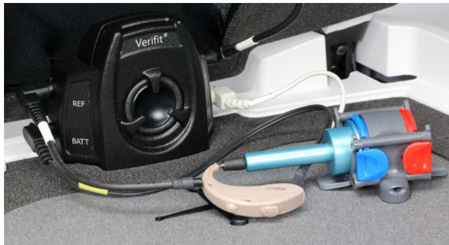
Positioning a BTE instrument for ANSI tests
