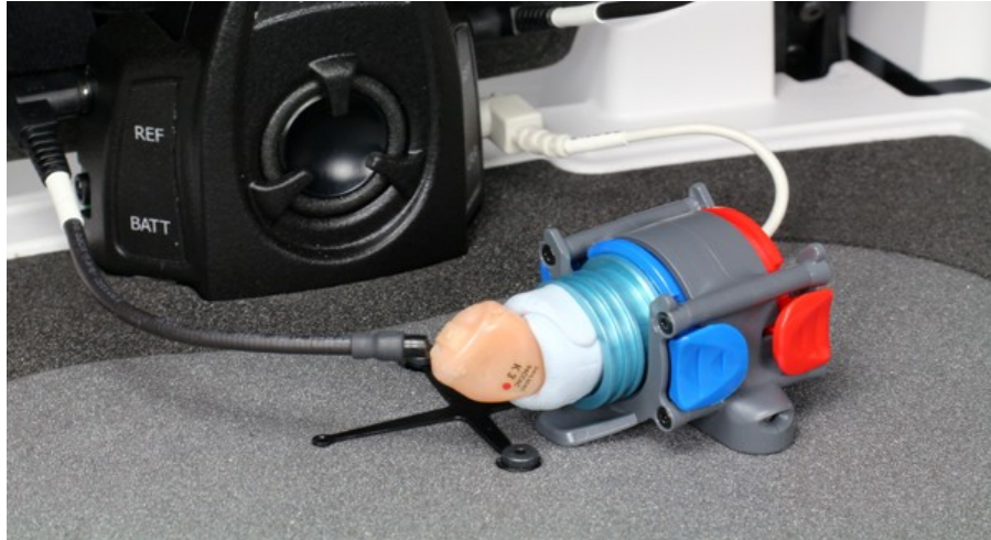
Positioning an ITE instrument for ANSI tests
